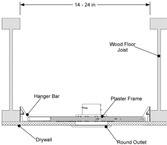
**Figure 1. Typical Installation**
